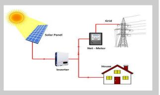
An assemblage of photovoltaic solar cells mounted on a frame that collects solar energy and converts it into sustainable energy is referred to as a solar panel. Each solar cell is built on a semiconductor material, often silicon. It is photovoltaic effect-sensitive and produces energy when exposed to sunlight as a result of this natural occurrence.
